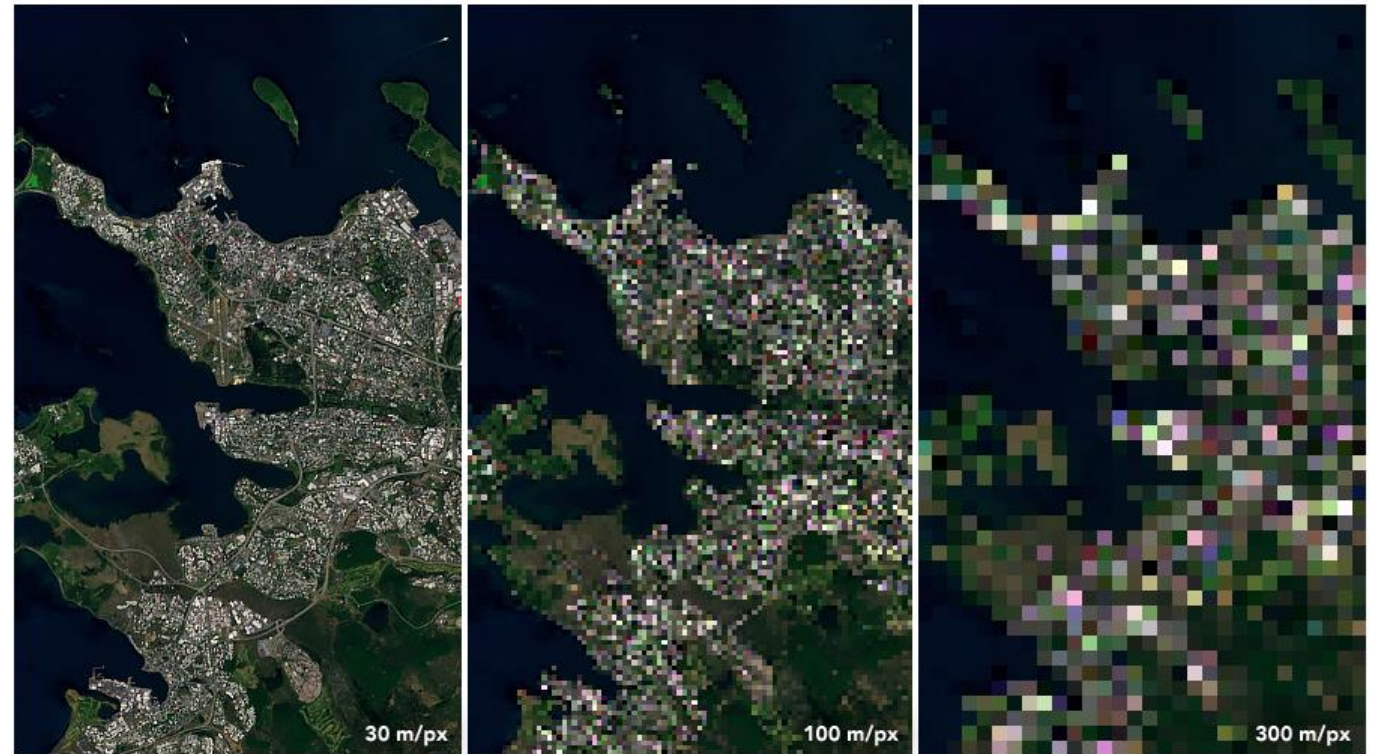
Landsat 8 image of Reykjavik, Iceland, acquired July 7, 2019, illustrating the difference in pixel resolution. Credit: NASA Earth Observatory.
